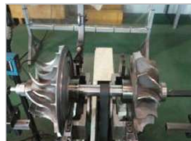
Carried out Dynamic Balancing Test
