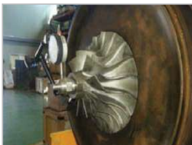
Measured Radial Clearance
